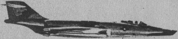
Republic F-105 Thunderchief USAF fighter bomber. Armed with vulcan cannon, a typical load: two 450 gallon fuel tanks and six 750lb. bombs.
