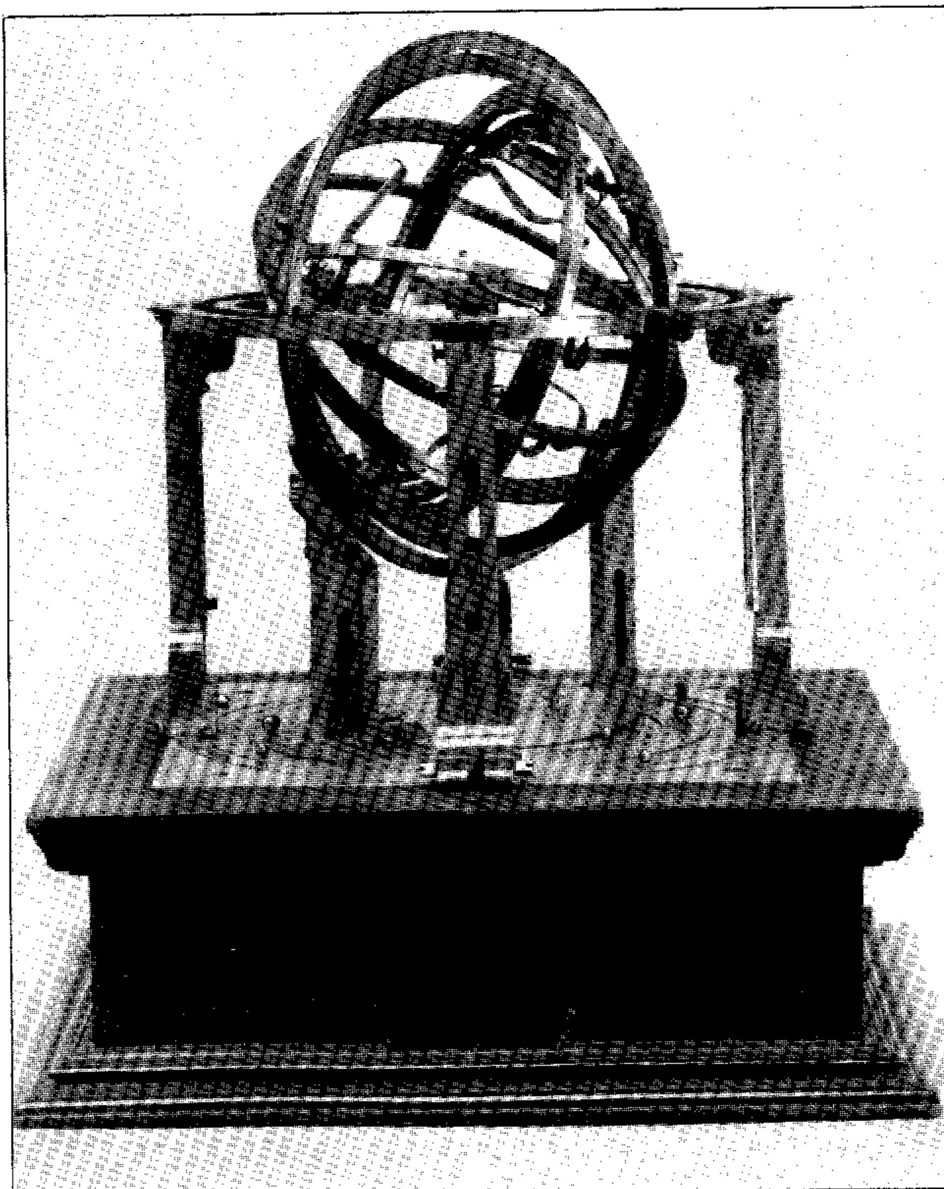
This armillary sphere from the sixteenth century enabled the accurate measurement of angles for use in calculations of distances to heavenly bodies.
