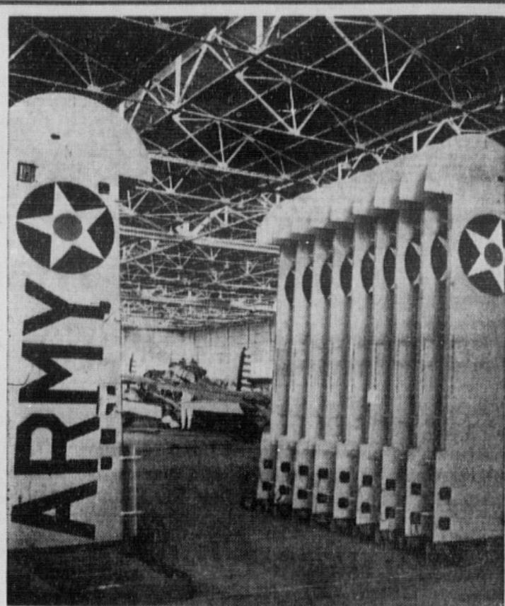
MASS PRODUCTION SPEEDS UP AT CALIFORNIA PLANE PLANT: Wing section of Army planes waiting completion in the Vultee Aircraft factory which is operating under the conveyor system which made the American automobile industry the most efficient in the world. In background is a fully assembled ship.
