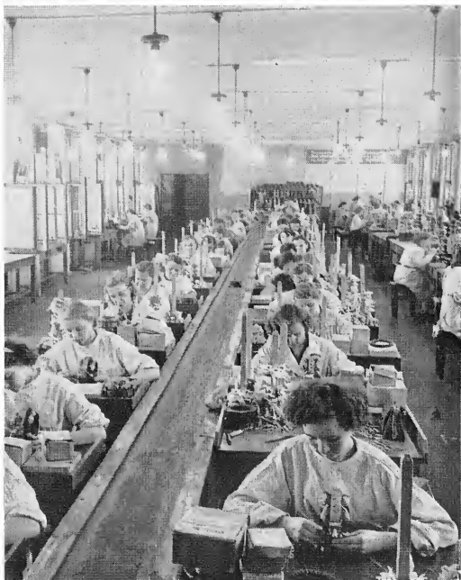
The women on the left are winding small electric motors for refrigerators and washing machines at the Elfa Factory, Vilnius.
