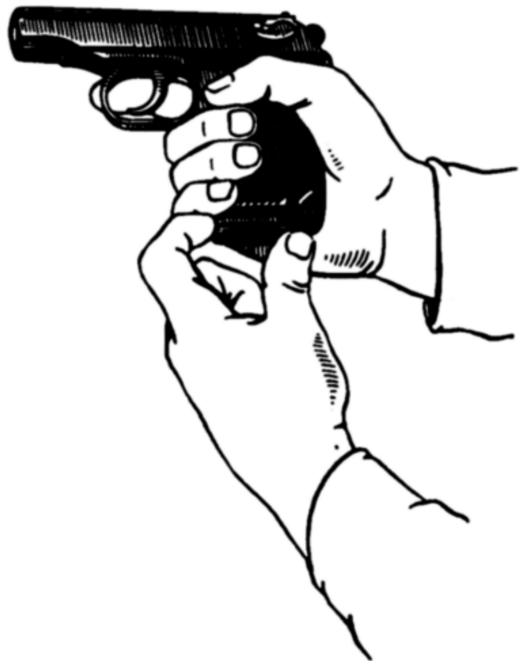
Fig. 3. Removing magazine from grip
