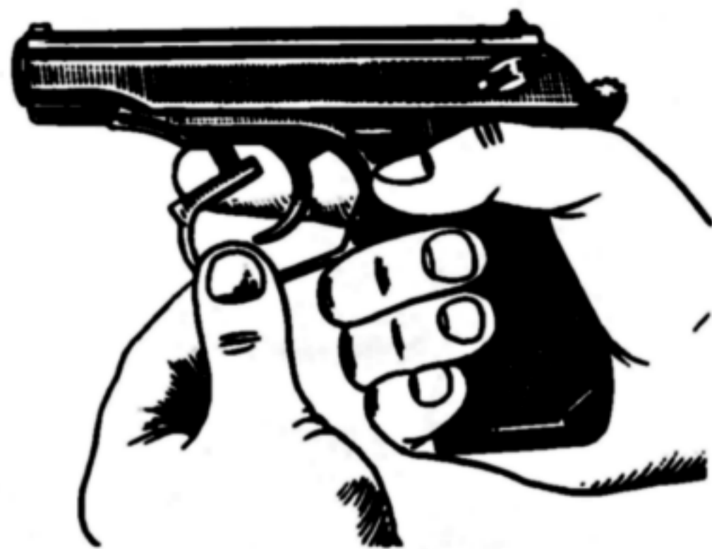
Fig. 4. Pulling down forward end of trigger guard
