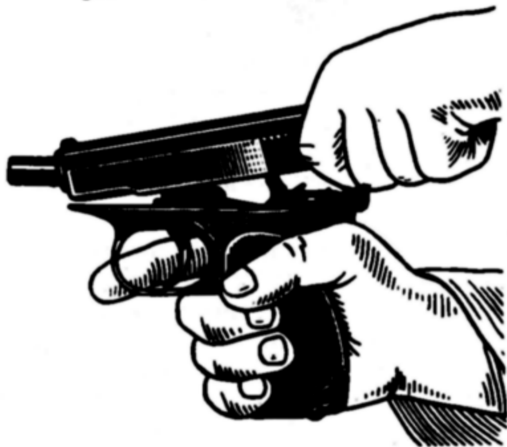
Fig. 5. Detaching slide from receiver
