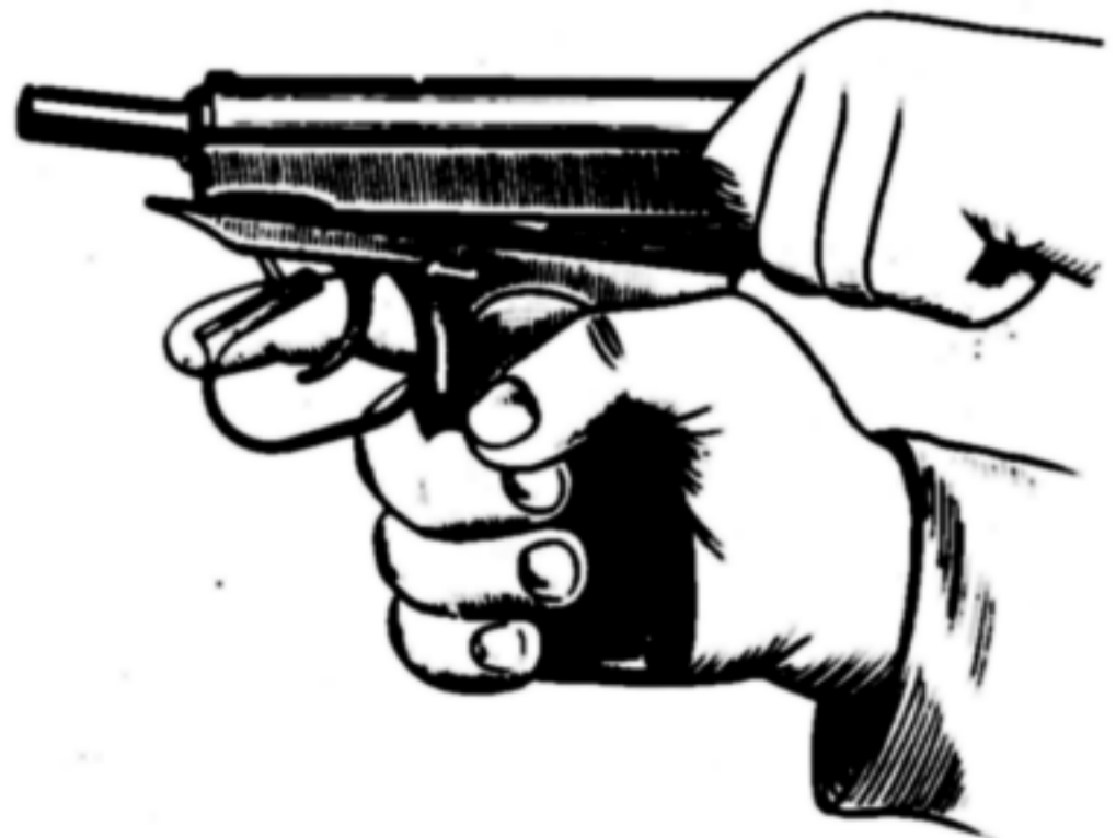
Fig. 6. Coupling slide to receiver
