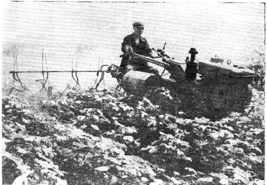
Mechanized sprayer made by the commune's farm machinery plant.
