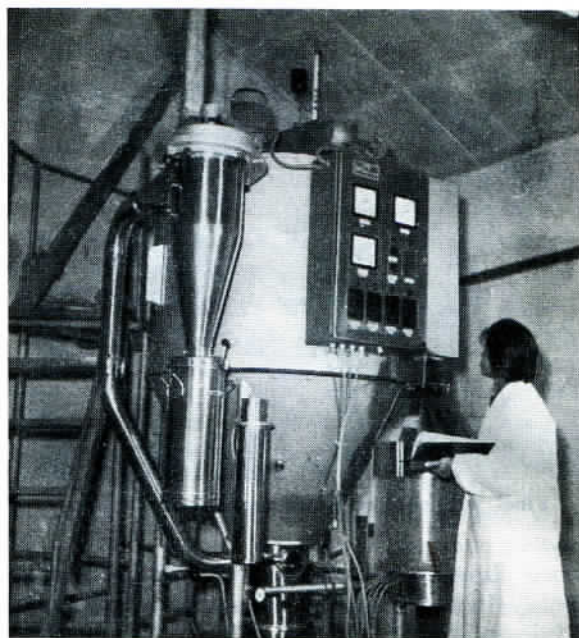
Spray-dryer imported from Denmark.
