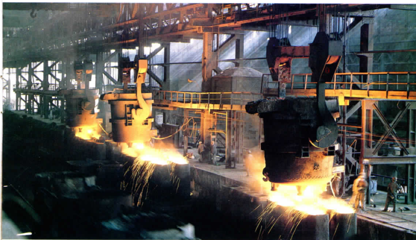
Workers at the No. 2 Steel Mill of the Anshan Iron and Steel Company pour steel ingots.
